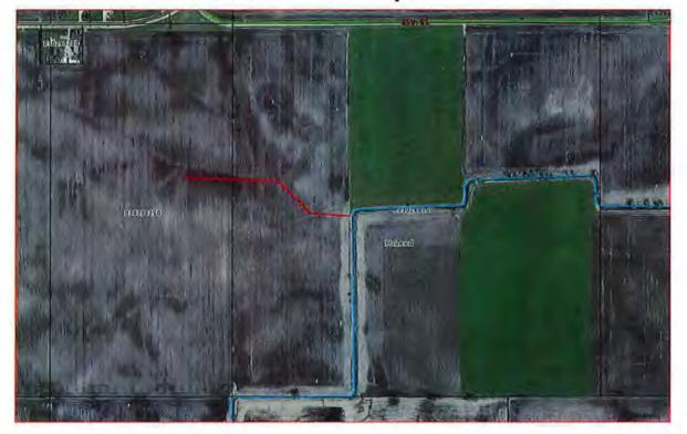
Ewert tiling scoped Branch 2 on CD #64 to see what condition the tile line is in. After viewing the video of the tile line, it was evident that it needed to be replaced. There are numerous locations in the line where the tile is cracked or broken, and places where obstructions limited the advancement of the camera. I recommend Branch 2 be replaced with dual wall cpe pipe. The line is highlighted in red.
