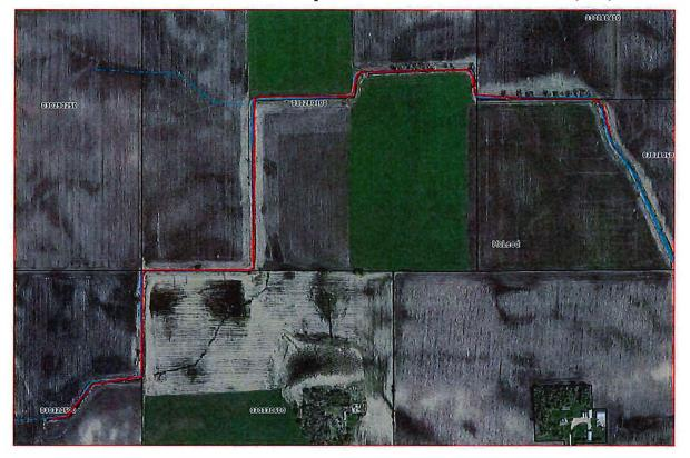
Met with Doug Benson regarding the condition of CD #64, the ditch has approximately 60 trees on the embankment and a couple close to the channel that need to be removed. The ditch will also need a clean out and some embankment improvements. I recommend that we start with tree removal this winter and then a ditch clean out this spring.
